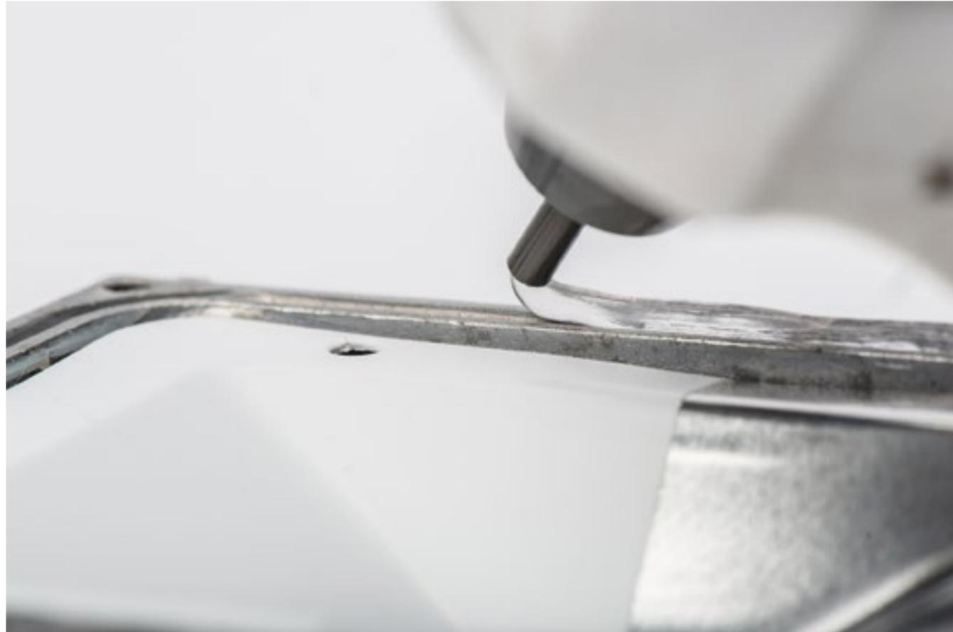
Hot-melt, neutral-cure sealants are intended for assembly, bonding, sealing, gasketing and other OEM applications that require instant adhesion and high green strength.<sup>1</sup>
