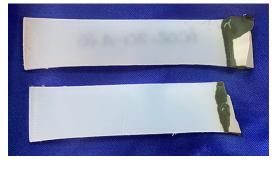
This image shows the adhesive bond is so strong that the nylon deforms and breaks
