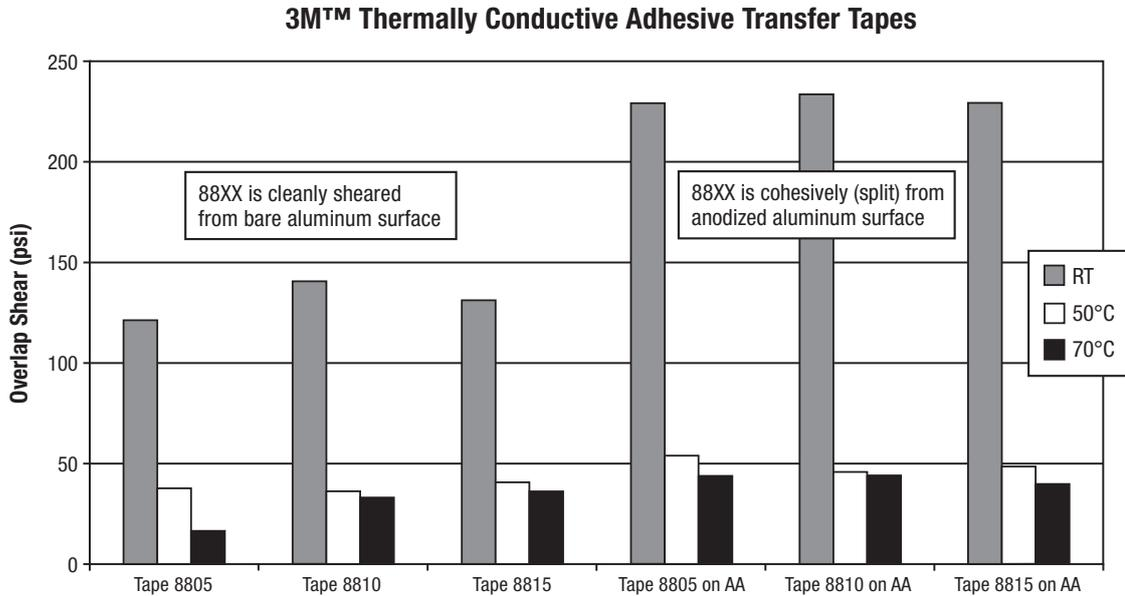
**Overlap Shear Heat Aged Properties:** (Test conditions: Test substrates are bare untreated aluminum, OLS speed is 0.5 in./min., adhesive cleanly removes from substrate surface during OLS test, 1 in.<sup>2</sup> test sample size, test at RT conditions after aging cycle complete, 3M Tape 8810).
