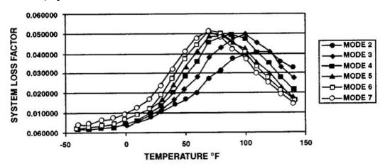
**Test Method:**The following data were obtained by doing a frequency sweep from 1 to 100 radians/sec (0.16 to 16 Hz) at 5 different temperatures: -20°, 10°, 0°, 10°, and 22°C. A 3 point bend geometry was used on the Rheometics RSA II. Time – temperature superposition was used to create the master curve for a reference temperature of 22°C.
