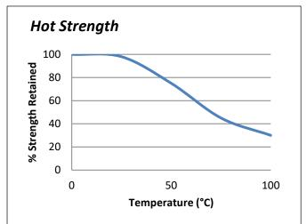
Fully cured lap shear specimens conditioned to pull temperature for 30 minutes before testing at temperature.
