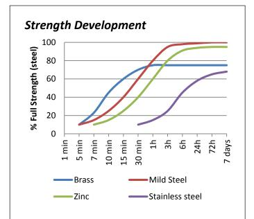
\*Cure times are typical at 23°C. Copper and its alloys will follow the faster cure while oxidised or passivated surfaces like stainless steel will tend towards the slower curve. Lower temperatures or large gaps will tend to extend the cure time. To reduce the cure time the use of Permabond A905, ASC10, or heat can be considered.
