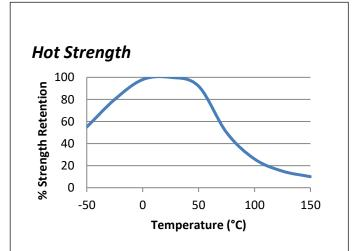
"Hot strength" shear strength tests performed on mild steel. 24hr cure at room temperature and conditioned to pull temperature for 30 minutes before testina.
