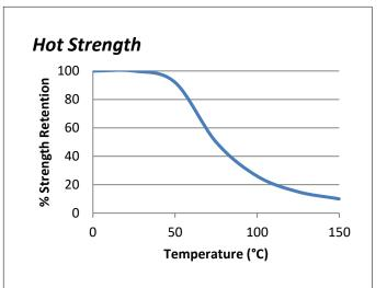
"Hot strength" shear strength tests performed on mild steel. Fully cured specimens  $conditioned\ to\ pull\ temperature\ for\ 30\ minutes\ before\ testing\ at\ temperature.$ TW42 can withstand higher temperatures for brief periods (such as for paint baking and wave soldering processes) providing the joint is not unduly stressed. The minimum temperature the cured adhesive can be exposed to is -40°C (-40°F) depending on the materials being bonded.
