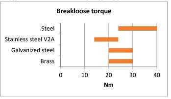
Breakloose torque on M10 bolts and nuts in Nm according to DIN 54454, free swimming without on-torque.
