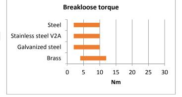
Breakloose torgue on M10 bolts and nuts in Nm according to DIN 54454, free swimming without ontorque.
