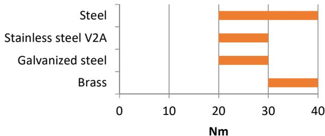
Breakloose torque on M10 bolts and nuts in Nm according to DIN 54454, free swimming without on-torque.
