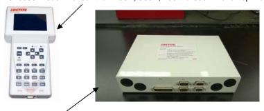
**2182205** EQ ACĆE D-Series Junction Box, 200D, 300D, 400D & 500D Robots. Provides a convenient connection point between robots and up to 8 external devices including all Loctite® dispensers, UV Wands, Loctite® light curtains, LED cure systems, Posi-Link™ Volumetric Dispensing System. Allows multiple systems integration simultaneously. This junction box accepts up to 8 inputs and 8 outputs, 24 VDC operation.
