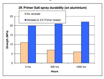
The graph above shows the use of Permabond 2K Primer on abraded aluminium surfaces bonded with a structural acrylic adhesive. The results of the salt spray aging test show improved durability.
