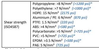
\*Substrate failure was observed.
