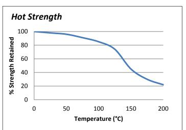
then conditioned to pull temperature for 30 minutes before testing. ES569 can withstand higher temperatures for brief periods (such as for paint baking and wave soldering processes) providing the joint is not unduly stressed. The minimum temperature the cured adhesive can be exposed to is -40°C (-40°F) depending on the materials being bonded.
