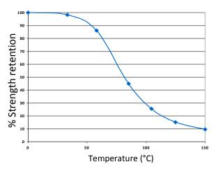
MT3808 can withstand higher temperatures for brief periods (such as for paint baking and wave soldering processes) providing the joint is not unduly stressed. The minimum temperature the cured adhesive can be exposed to is -40°C (-40°F) depending on the materials being bonded.
