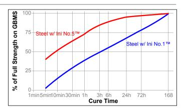
The graph below shows the shear strength developed with time on PVC lap shears and tested according to ISO 4587 Activator Ini No.1<sup>™</sup> or Ini No.5<sup>™</sup> applied to one surface
